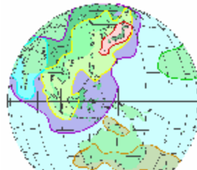
Covered area by JCSAT-3 satellite Yellow – Ku-band (Asia zone) Purple – C-band (Asia zone)
